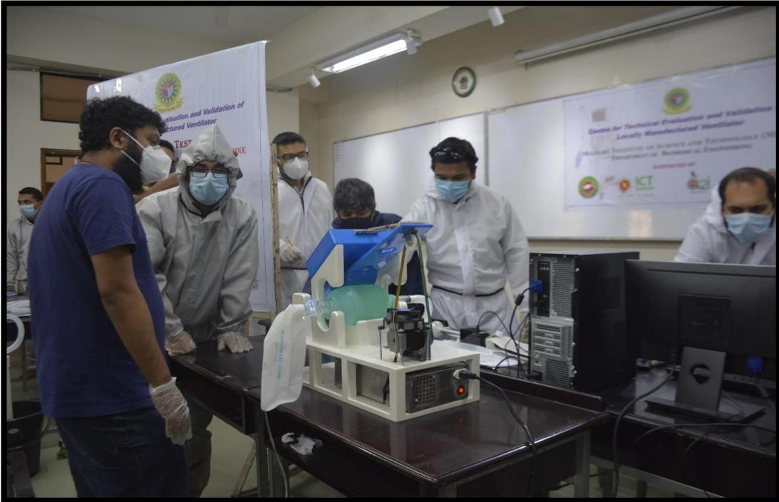
**Testing of Ventilator from Bangladesh Machine Tools Factory (BMTF)**
